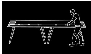
tile should be kept on flat support while cutting, do not keep any hollow gaps underneath the tile.
