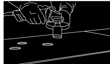
making holes on porcelain tiles by external round-cut machine with minimum thickness of 11mm.
