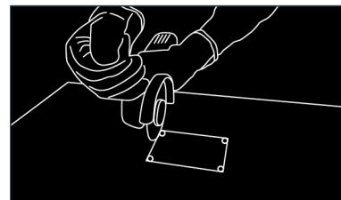
making I-shape and angled cuts on porcelain tiles with cnc or water-jet machines and even manual that should make rounded-off edge to protect the tiles from breaking.
