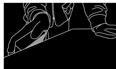
for finishing the sides of porcelain tiles abrasive pads can also be used.
